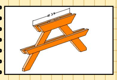
Legs + seat beams + top beams assembled.
