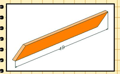
The next step requires the most difficult measurement and cutting in the entire project. Using a combination square, measure back 1-3/4" along the mitre cut, from the pointy end of the board. Mark a line perpendicular to the mitre cut, which should end at the edge of the board, 1-3/4" across. Mark and cut these points off on all eight ends of the four legs. This completes cutting of the legs. You should have four legs that look like this:
